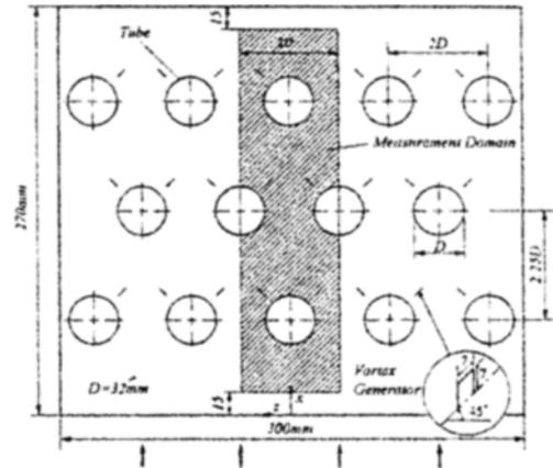
Fig. 1 Schematic of fin-circular tube heat exchanger model
