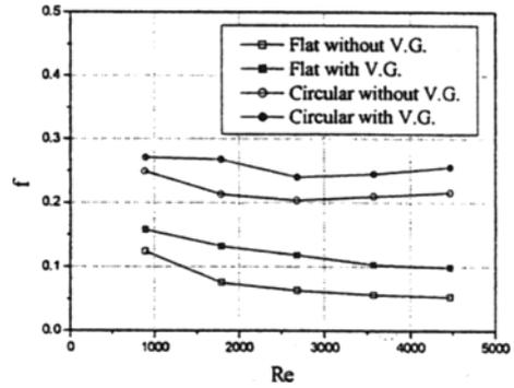
Fig. 9 Comparison of apparent friction factors for four types of heat exchanger
