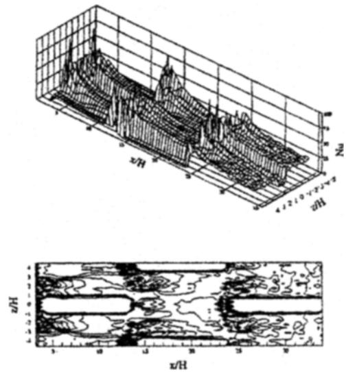
Fig. 7 Distribution of local Nusselt number for fin-flat tube heat exchanger with vortex generators
