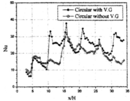
**Fig. 4** Comparison of spanwise-averaged heat transfer for fin-circular tube heat exchanger
