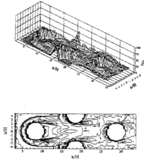
Fig. 2 Distribution of local Nusselt number for fin-circular tube heat exchanger without vortex generators
